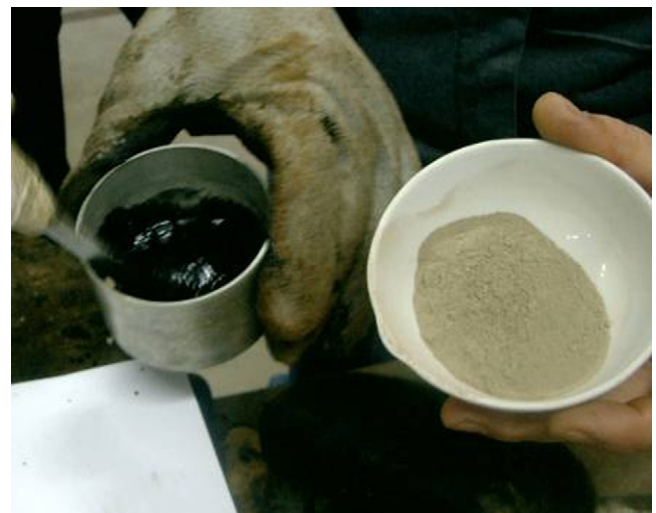
Fig. 5. Preparation of the delta ring and ball sample.
